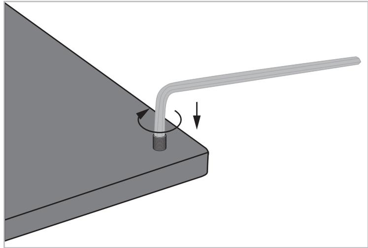
Screw in the adjustable foot flush-mounted from above with the supplied allen key.
