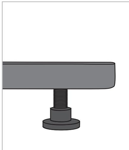
Side view of base plate / adjustable foot
