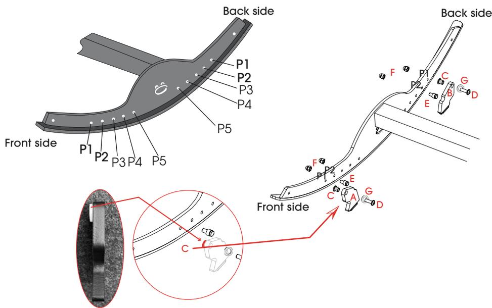
1. Screw in hand-tight one foot (A/B) each into the runners from the inside (at the 4 positions P1) using a round-headed bolt (D) and a spring washer (G) (note "front" and "rear" here).
